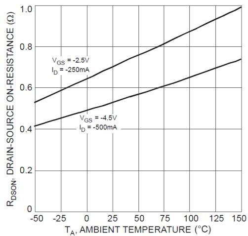
Fig. 6 On-Resistance Variation with  $T_A$
