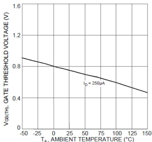
Fig. 7 Gate Threshold Variation vs.  $T_A$
