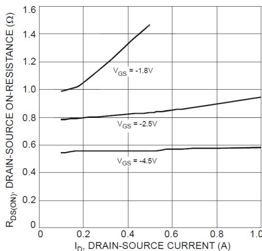
Fig. 3 Typical On-Resistance vs.  $I_D$  and  $V_{GS}$
