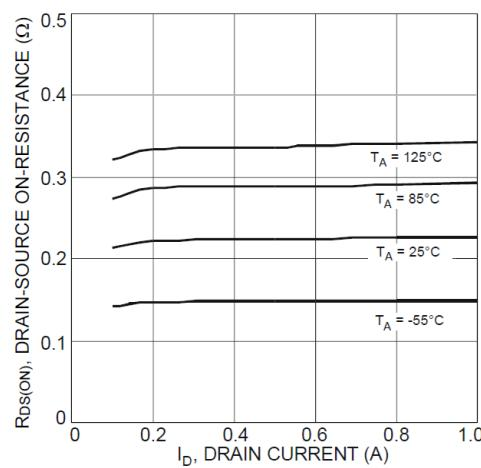
Fig. 4 Typical Drain-Source On-Resistance vs.  $I_D$  and  $T_J$
