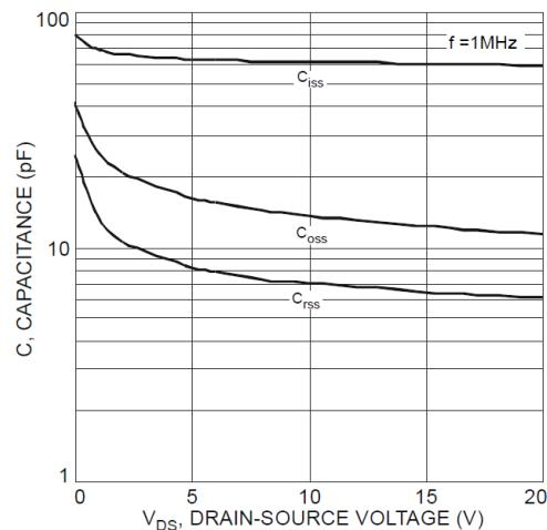
Fig. 9 Typical Capacitance
