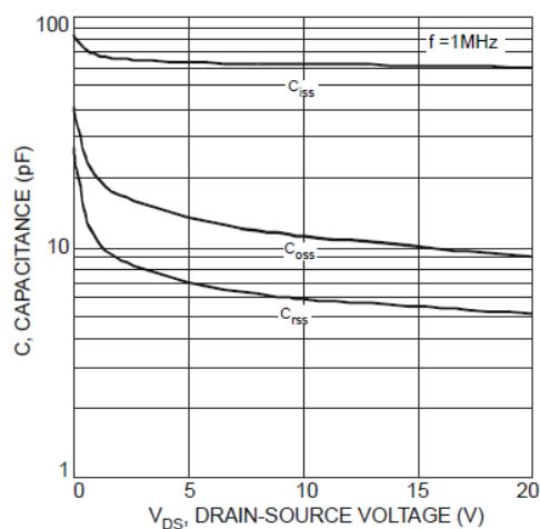
Fig. 9 Typical Capacitance
