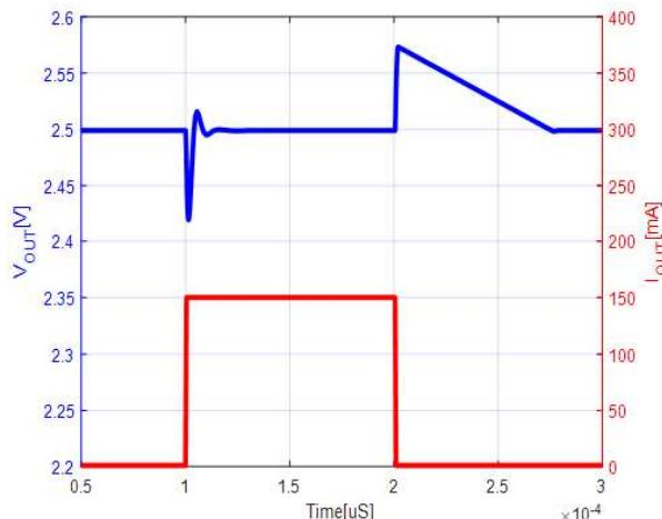
$I_{\text{OUT}}=50\text{mA}\sim 100\text{mA}, T_r=T_f=0.5\mu\text{s}, C_{\text{in}}=C_{\text{out}}=1\mu\text{F}$
