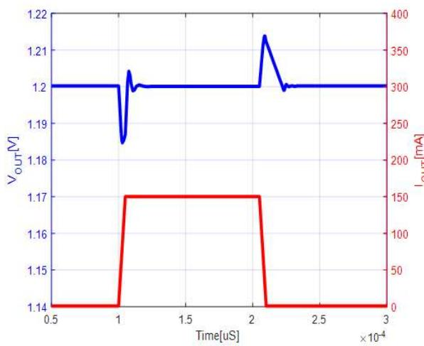
$I_{\text{out}}=50\text{mA}\sim100\text{mA}, T_r=T_f=5\mu\text{s}, C_{\text{in}}=C_{\text{out}}=1\mu\text{F}$
