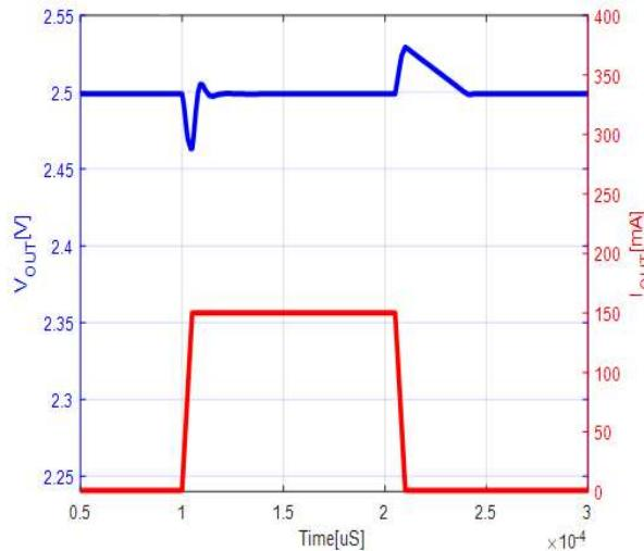
Iout=50mA~100mA, Tr=Tf=5 $\mu\text{s}$ , Cin=Cout=1 $\mu\text{F}$
