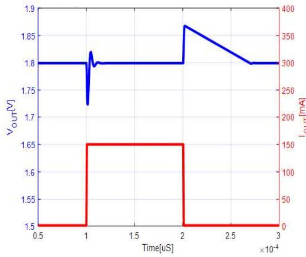
$I_{\text{OUT}}=50\text{mA}\sim 100\text{mA}, T_r=T_f=0.5\mu\text{s}, C_{\text{in}}=C_{\text{out}}=1\mu\text{F}$
