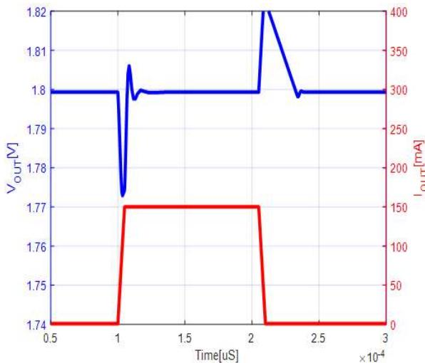
$I_{\text{out}}=50\text{mA}\sim100\text{mA}, T_r=T_f=5\mu\text{s}, C_{\text{in}}=C_{\text{out}}=1\mu\text{F}$
