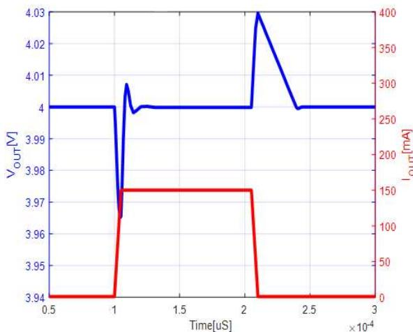
Iout=50mA~100mA, Tr=Tf=5 $\mu\text{s}$ , Cin=Cout=1 $\mu\text{F}$
