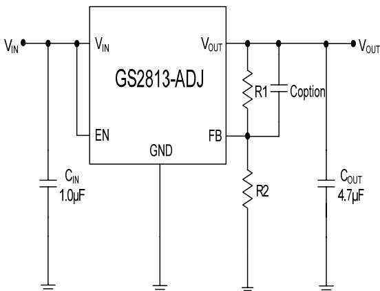
Figure2. ADJ Voltage Operation
