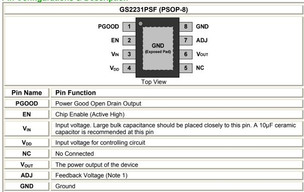
**Note1.** For adjustable version parts a resistor divider on this pin sets the output voltage according to the relation:  $V_{OUT}=0.8 \text{ X (R1 + R2)} / \text{R2}$ .
